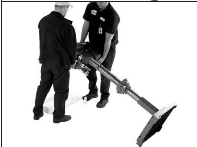
Figure 12. Tilting drill press upright.
